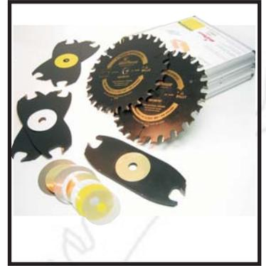
This new and improved dado set will produce flat bottom grooves with splinter free edges in all natural woods. The blades feature 24 teeth with thick C4 carbide for guaranteed sharp edges and longer tool life. Fully versatile, this dado set can be set from 1/4" to 1" widths at 1/16" increments. The set also includes **FIVE** chippers (rather than the standard four), including a 3/32" chipper for smaller increments to accommodate actual wood sizes.
